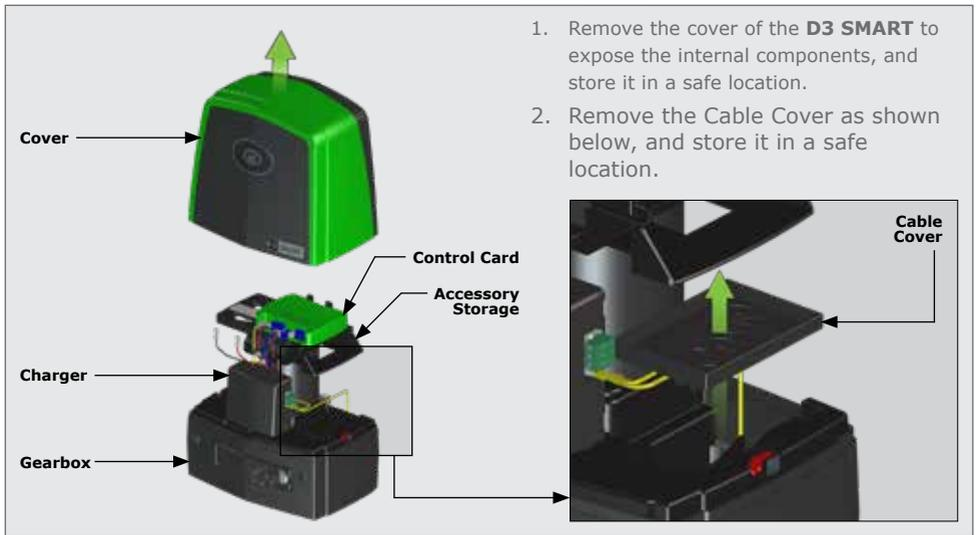
1. Remove the cover of the **D3 SMART** to expose the internal components, and store it in a safe location.
