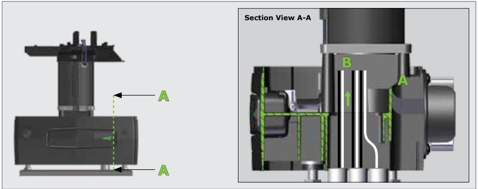
FIGURE 44. CABLE ROUTING FOR RETRO-FITS WITH SHORTER CABLES
